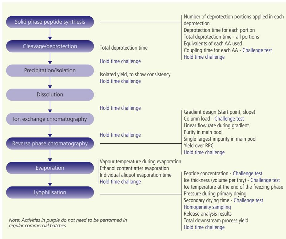
Figure 2 - Non-exhaustive list of parameters monitored during the manufacture of a peptide process performance qualification batch
