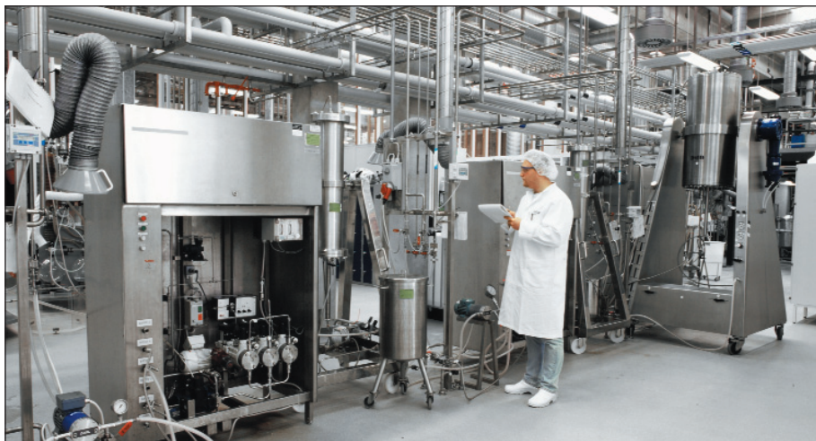
As project requirements grow and lot sizes increase, large-scale purification equipment is used for the manufacture of GMP peptides
