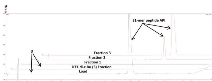
Figure 4. Removal of the adduct **3** from a solution of a 31-mer peptide API by RP-HPLC. Stationary phase: silica C18; mobile phase: 10 mM phosphate buffer pH 7.5/MeCN. Note that this RP-HPLC run was not aimed at increasing the purity of the peptide API.
