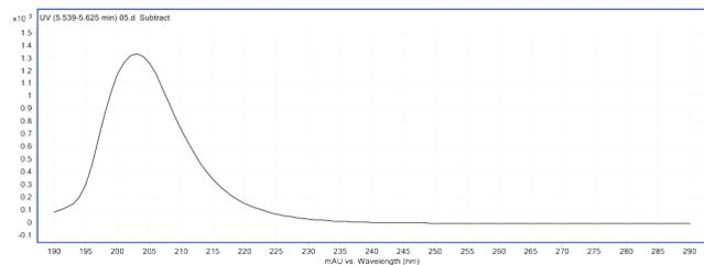
Figure 2. UV spectrum of a low MW impurity detected in the solutions of a 31-mer peptide API.
