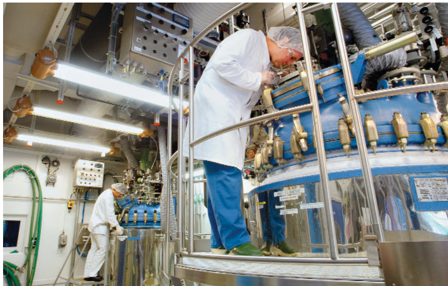
WET OR DRY PolyPeptide uses solution-phase methods, shown here, and solid-phase techniques to synthesize peptides at its Torrance, Calif., facility.
